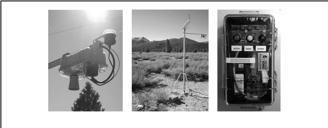
**Figure 6.1:** A Snowcloud Sensor Node (L,C) and Harvester Device (R).
