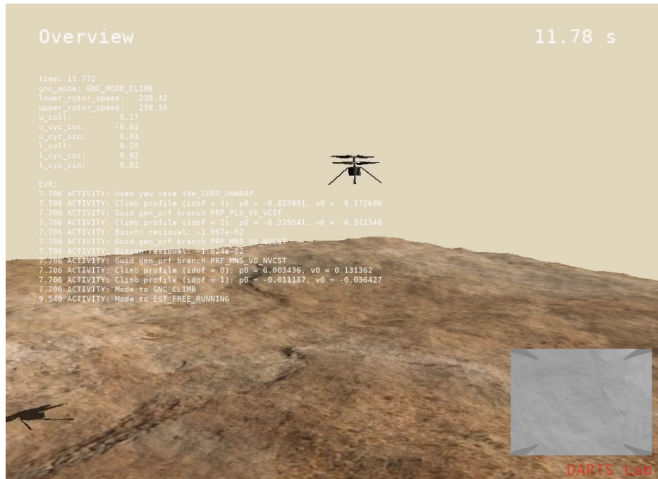
Fig. 10 Screenshot from a simulated flight in HeliCAT. The view from the navigation camera is shown in the bottom right corner.
