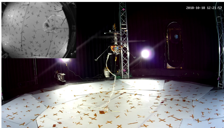
Fig. 5 EDM-1 during a recent flight test, using only onboard sensors for navigation. The view from the navigation camera can be seen in the upper left-hand corner.
