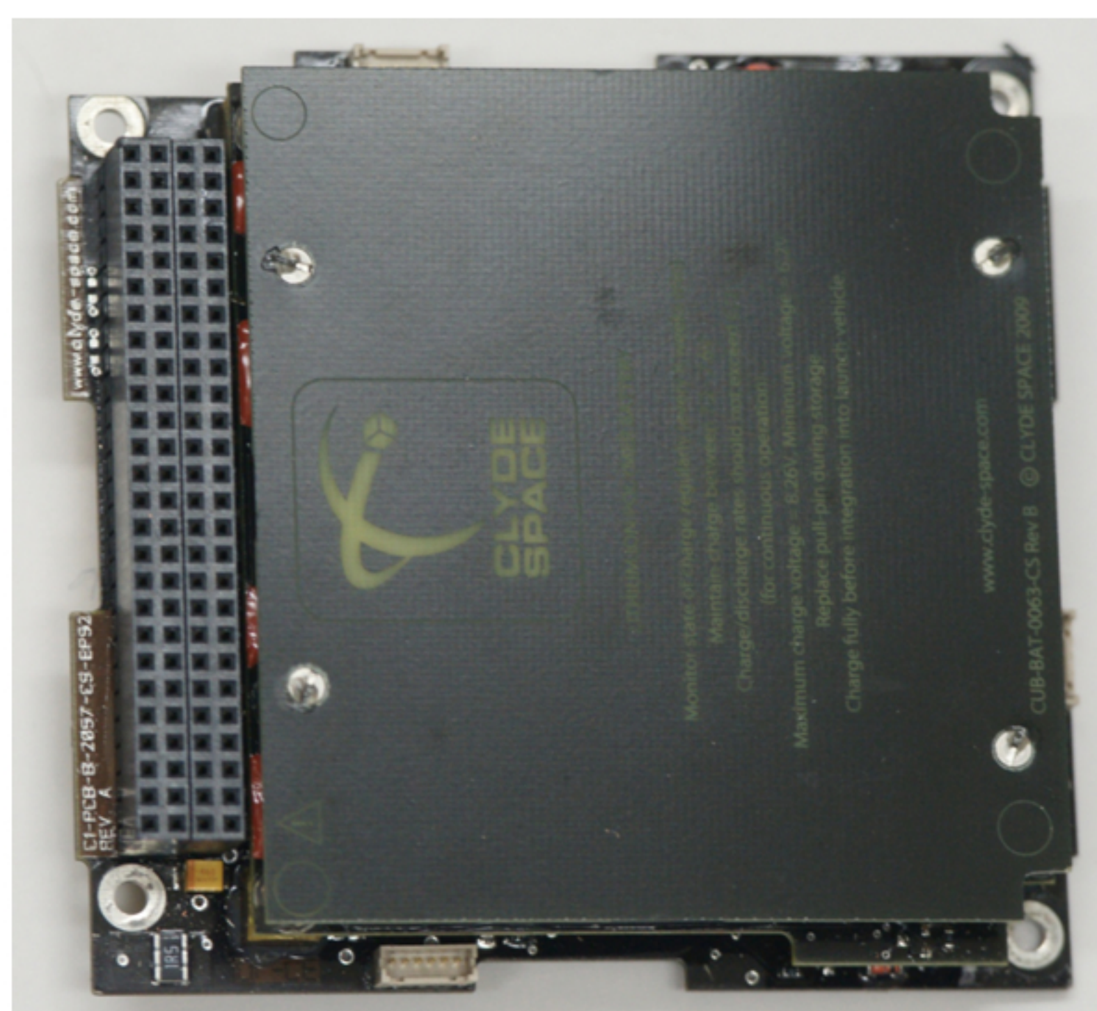
Clyde Space EPS & Battery
